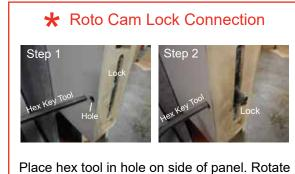
to activate lock & secure panels together.
